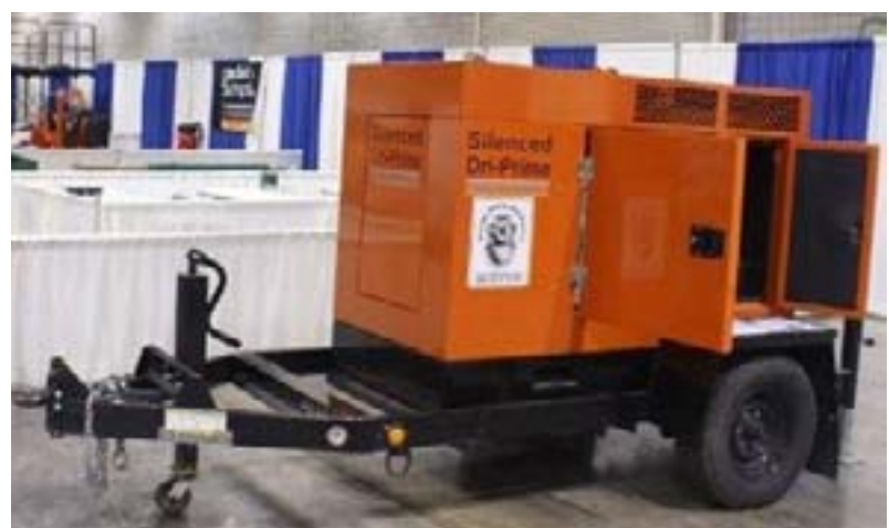
CD100M Critically Silenced 4" Dri-Prime Pump
