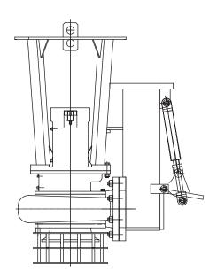
The Heidra HS200SG is a versatile, 8" (200mm) hydraulic submersible pump capable of passing large solids up to 3-1/8" (79mm), stringy materials and slurries. A remotely-operated slurry gate allows the pump to act as a mixer, ideal for pumping thick, viscous, solids-laden sludges, such as those found in WWTP digesters, environmental clean-ups and API separators at refineries.
